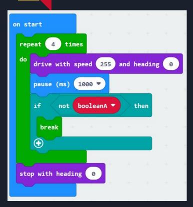
In the code to the left, an extremely simple loop will run 4 times. This code highlights how simple loops can be. If you explore under the "Loops" tab in MakeCode, you will see that this is simply the first example of a loop, with *while* and *for* loops also being present. Try out some of them! As a part of the code, though, there is an *If* statement with a *break* in it.
