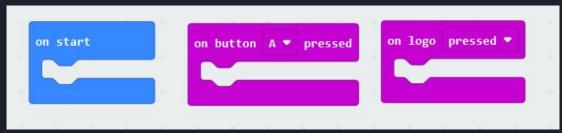
Notice that each input makes its own block, that means you can have the micro:bit do things only when it receives certain inputs, like a button being pressed!
