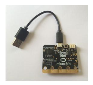
Now that the micro:bit has been connected to the computer, the last step will always be to download the program to the micro:bit. Following any of the lessons provided, students should be able to write a program in *MakeCode*. Once they are ready to test it on the micro:bit, all that needs to be done is to click the "Download" button in *MakeCode* (below), located in the bottom-left corner. *MakeCode* should automatically compile and write the code to the micro:bit.
